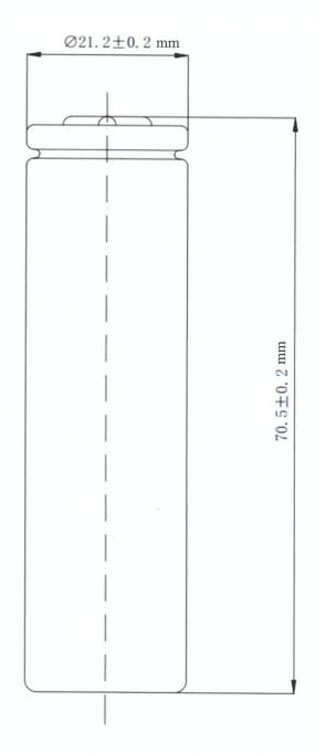
With thermoplastic sleeve 带热缩套
